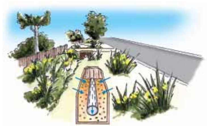
Above: Illustration showing cutaway of swale
